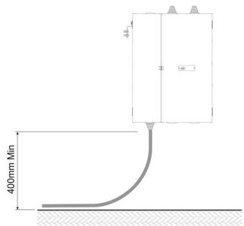
3: Mark then drill the mounting surface with an appropriately sized drill bit such that a Rawlplug insert for an M8 or M10 stud or setscrew can be inserted. If using a stud, it should protrude approximately 25mm from the mounting surface. A flat washer should be under the bolt head (or nut if using a stud) to spread the clamping force.
