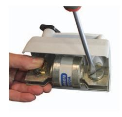
5: Using the appropriate PPE, install the fuse handle and tighten both thumbscrews as tight as is comfortably possible. This corresponds to a torque of approximately 7-8Nm.
