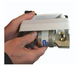
Ensure both clamps are in their fully released position by backing off the thumbscrews.
