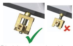
4 : Tighten both retention screws down to their abutment shoulders.
