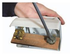
3 : Place a BS88 fuse with 92mm fixing centres over the brass spigots which form part of the clamping wedges. Ensure that the fuse link is attached as shown with its open slot uppermost.
