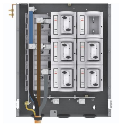
6 : Check that the groove in the grommet locates correctly in the 'U' slot in the cabinet when the cable is in it's final position.
