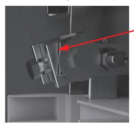
Note angle of the neutral connector to ensure the N conductor lays flat.
