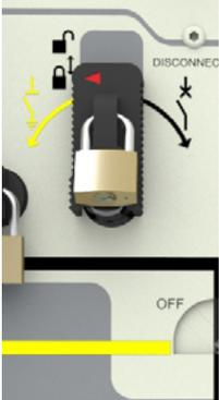
The mechanism consists of one operating shaft and one selector. The operating shaft is used for switching ON / OFF (Mains or Earth) and the selector is used for selection of the Mains or Earth positions. It is impossible to simultaneously close the Load Break Switch / Circuit Breaker and the Earth switch.
