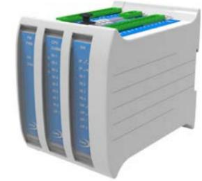
The Gemini 3 Mini is part of the Gemini 3 Platform providing advanced monitoring and control for medium voltage switchgear. Switch control is achieved locally with the HMI module (common to the Gemini 3 Modular family), via hard-wired inputs, or remotely over a communication link.
