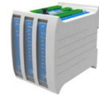
The Gemini 3 Mini is the latest addition to Lucy Electric's Gemini family of RTUs. The Gemini 3 Mini range comprises small composite DIN rail sub-assemblies providing the optimum suitability for overhead and ground mount switchgear. It is designed to monitor and control switchgear used in medium voltage secondary distribution applications. Switch control is achieved locally with the HMI (common to the Gemini 3 Modular RTU) or remotely over a communication link.
